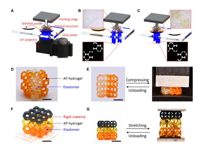
Multimaterial 3D printing hydrogel with other polymers. (A) Illustration of the DLP-based multimaterial 3D printing apparatus. (B and C) Processes of printing elastomer and hydrogel structures, respectively. (D) Snapshot of a diagonally symmetric Kelvin form made of AP hydrogel and elastomer. (E) Demonstration of the high deformability of the printed diagonally symmetric Kelvin form. (F) Snapshot of a printed Kelvin foam consisting of rigid polymer, AP hydrogel, and
