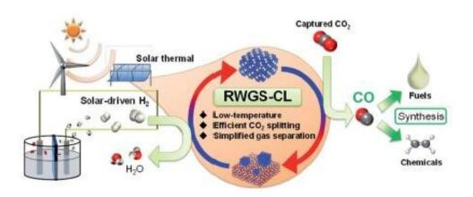
A chemical-looping version of the reverse water-gas shift reaction (RWGS-CL) can help convert carbon dioxide to carbon monoxide at much lower temperatures without undesirable byproducts, enabling a simple gas separation Credit: Yasushi Sekine from Waseda University
