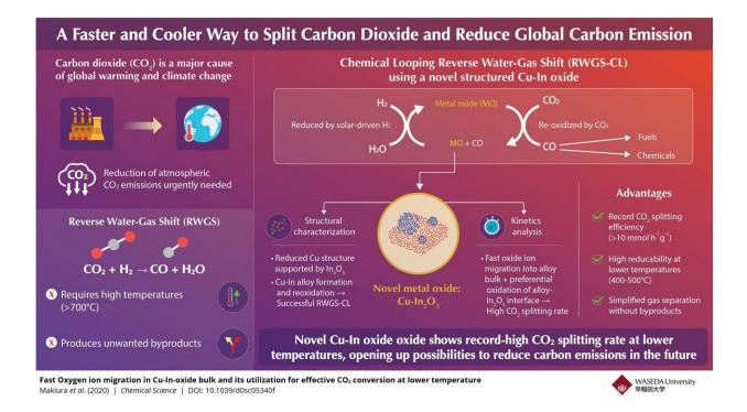
A record-high  $CO_2$  conversion rates at relatively low temperatures in a modified chemical-looping version of RWGS using a novel copper-indium oxide Credit: Waseda University
