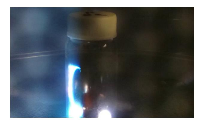
In a microwave oven, sparks are generated inside a glass vial containing coal powder and copper foil as part of an experiment by UW researchers. They successfully converted the coal powder to nano-graphite, demonstrating a novel and inexpensive coal-conversion technology. Credit: UW Photo
