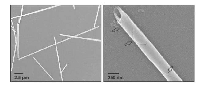
Electron micrographs give a detailed view of the new nanomaterial. Arrows indicate layers that form in the tubes, leading the researchers to hypothesize that the sheets form tubes by scrolling in at the corners. Credit: Emory University
