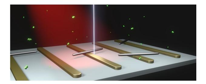
Depiction of the experimental setup where palladium nanorods lie atop gold nanobars. In this image, an electron beam is directed at the sample to watch the catalytic interactions between the hydrogen molecules (in green) and the palladium catalyst. The light driving the illumination is shown in red. Credit: Katherine Sytwu
