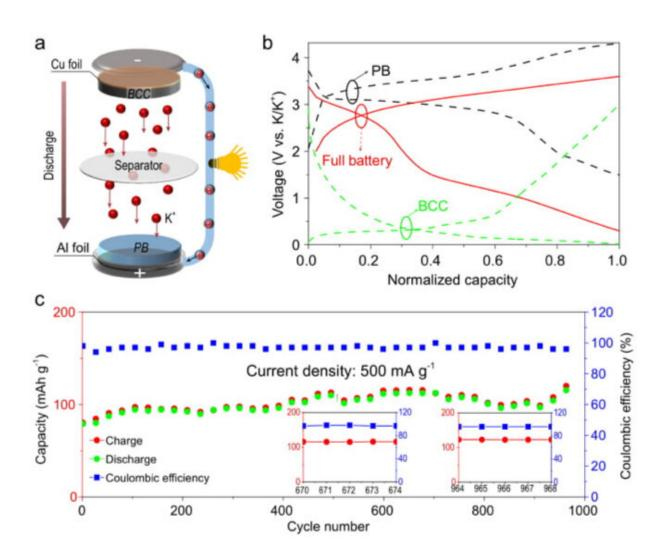
(a) Schematic illustration of the K-ion full battery based on the as-prepared BCC and Prussian Blue (PB). (b) Charge-discharge profiles of the half battery and full battery. (c) Cycling stability at 500 mA g-1. Credit: Science China Press
