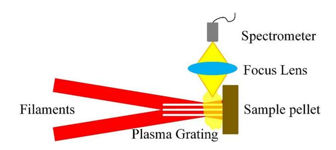
Experimental schematic of plasma grating induced breakdown spectroscopy, . Credit: doi 10.1117/1.AP.2.6.065001
