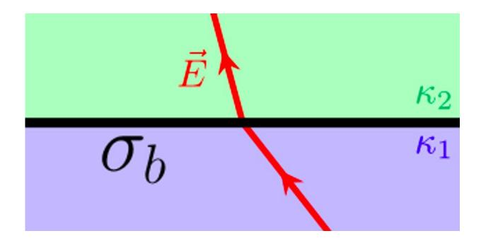
A simplified version of Fig. 1.(a) from the researchers' paper. Caption: When an electric field  $(\vec{E}')$  is incident on the interface (black line) between two materials (blue and green regions) with distinct permittivity values ( $\kappa_1$  and  $\kappa_2$ ), a surface bound charge ( $\sigma_b$ ) forms on that interface. Credit: Prentki et al.
