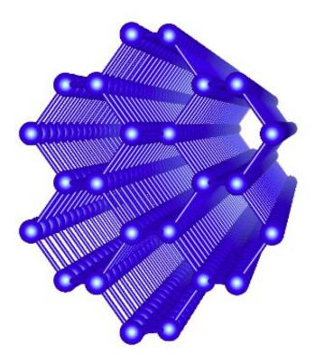
Image of one of the silicon nanowires that Prentki simulated in his work. Each sphere represents a silicon atom, and each bar represents an atomic bond between two neighboring silicon atoms. Credit: Prentki et al.
