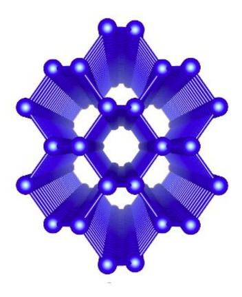
Image of one of the silicon nanowires that Prentki simulated in his work. Each sphere represents a silicon atom, and each bar represents an atomic bond between two neighboring silicon atoms. Credit: Prentki et al.
