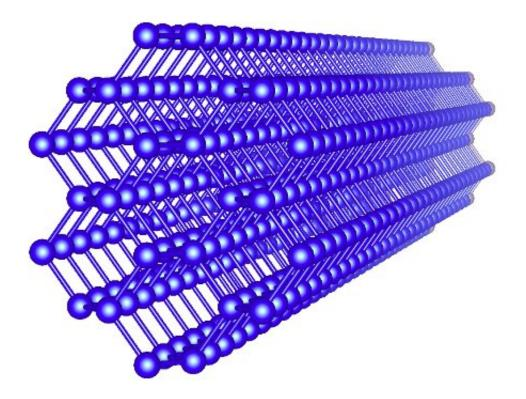
Image of one of the silicon nanowires that Prentki simulated in his work. Each sphere represents a silicon atom, and each bar represents an atomic bond between two neighboring silicon atoms. Credit: Prentki et al.
