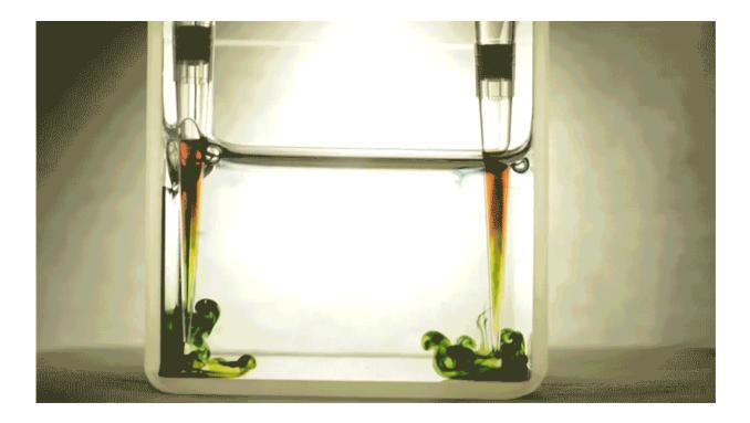
Here, dyes are used to reveal the concentration levels of carbon dioxide in the water. Green shows areas where the carbon dioxide is more concentrated, and blue shows areas where it is depleted. The green region at left shows the carbon dioxide staying concentrated next to the catalyst, thanks to the gas-attracting material. Credit: Varanasi Research Group
