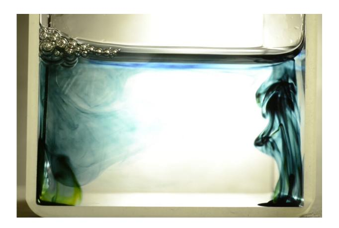
Dyes are used to reveal the concentration levels of carbon dioxide in the water. On the left side is a gas-attracting material, and the dye shows the carbon dioxide stays concentrated next to the catalyst. Credit: Varanasi Research Group
