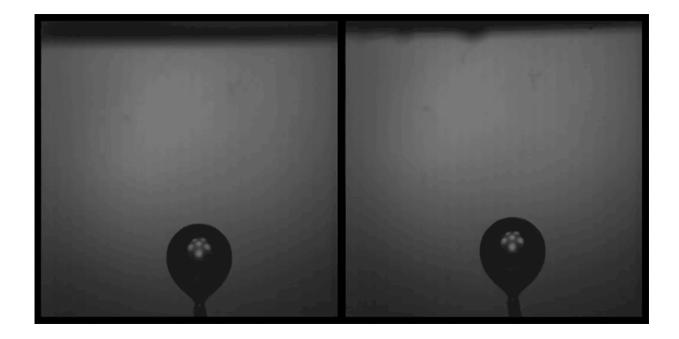
On the left, a bubble strikes a specially textured gas-attracting surface, and spreads out across the surface, while on the right a bubble strikes an untreated surface and just bounces away. The treated surface is used in the new work to keep the carbon dioxide close to a catalyst. Credit: Varanasi Research Group
