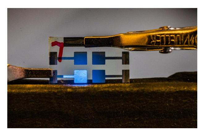
Blue light-emitting diodes based on halide perovskites. Credit: Thor Balkhed
