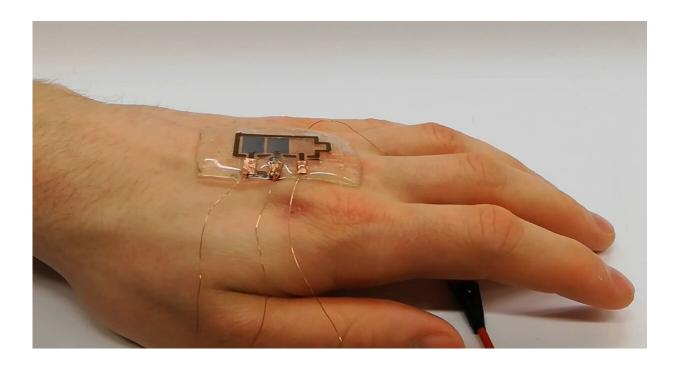
Thanks to its flexibility and adhesion, the biodegradable display can be worn directly on the hand. Credit: Manuel Pietsch, KIT
