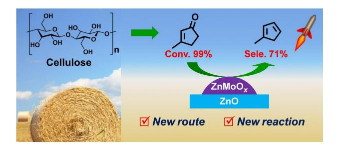
Direct hydrodeoxygenation of MCP to MCPD on the partially reduced Zn-Mo oxide catalyst. Credit: DICP
