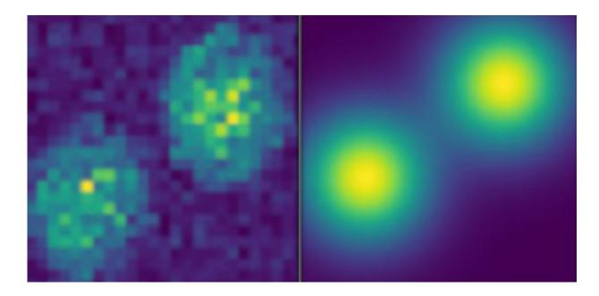
At left: Experimental PASSI (photon avalanche single-beam super-resolution imaging) images of thulium-doped avalanching nanoparticles separated by 300 nanometers. At right: PASSI simulations of the same material. Credit: Berkeley Lab and Columbia University
