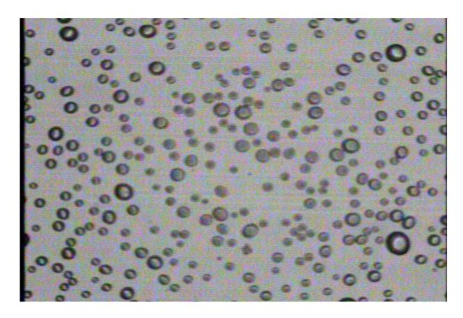
Supercooled liquid cloud droplets in the lower troposphere over the ice-free Arctic Ocean obtained by a HYdrometer VIdeo Sonde (HYVIS) observation on 22nd September 2014. Credit: Inoue J. et al. (2021)
