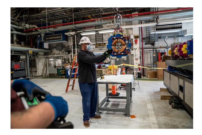
Driver/Rigger Brian McFadden uses a crane to lift a 660-pound quadrupole magnet, the final magnet to complete the first practice assembly for the upgrade of the Advanced Photon Source. Credit: JJ Starr/Argonne National Laboratory
