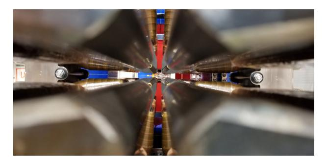
This image shows the path the electron beam will take through the center of the focusing and bending magnets as it circulates around the upgraded APS storage ring. Each of the 1,321 magnets that will make up the storage ring must be aligned with its neighbors to within half the width of a human hair. Credit: Ken Volin/Argonne National Laboratory
