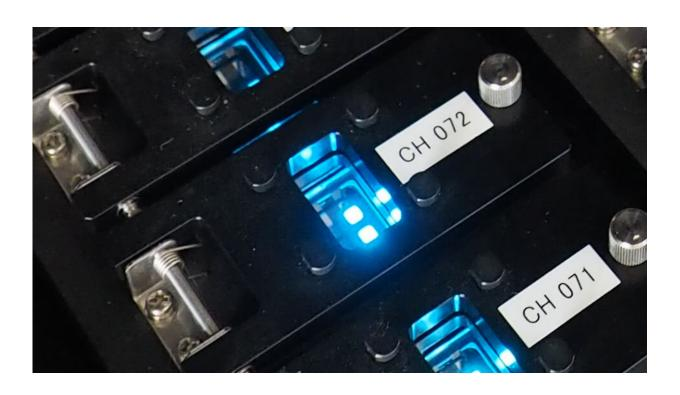
Highly efficient, pure-blue organic light-emitting diodes (OLEDs) developed by researchers at Kyushu University in Japan are being tested to measure their lifetime. Based on hyperfluorescence, which uses a two-molecule process to emit light, the OLEDs emit pure-blue emission and exhibit significantly improved lifetimes compared to other highly efficient devices, all without using expensive metal atoms. Credit: Masaki Tanaka, Kyushu University
