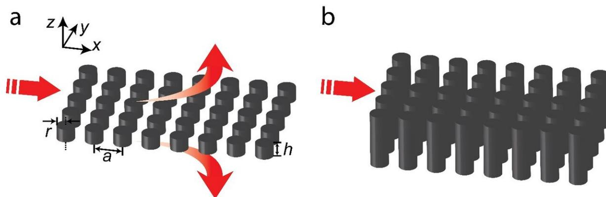
a, Zero-index PhC slab without BICs. A photonic dipole mode forming the zero index results in out-of-plane radiation, dramatically increasing the propagation loss of the material. b, Zero-index PhC slab with a BIC. At a particular height, all the upward/downward out-of-plane radiation destructively interferes. Credit: Tian Dong, Jiujiu Liang, Philip Camayd-Muñoz, Yueyang Liu, Haoning Tang, Shota Kita, Peipei Chen, Xiaojun Wu, Weiguo Chu, Eric Mazur, and Yang Li
