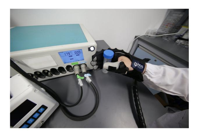
NUS researchers have developed wireless, ultra-thin and battery-free strain sensors that are 10 times more sensitive than conventional technologies. These light-weight strain sensors can be incorporated into rehabilitation gloves to improve their sensitivity and performance. Credit: National University of Singapore
