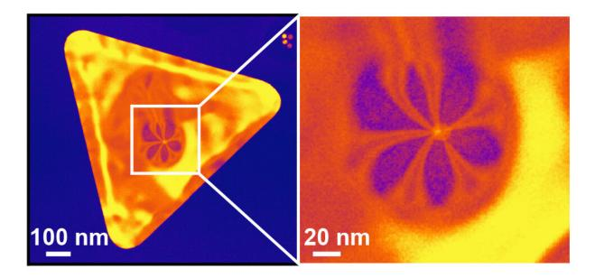
A transmission electron microscope image by Rice University scientists shows a silver nanoplate deformed by a particle, forming flower-shaped stress contours in the material that indicate a bump. Changing the shape of the material changes its electromagnetic properties, making it suitable for catalysis or optical applications. Credit: The Jones Lab/Rice University
