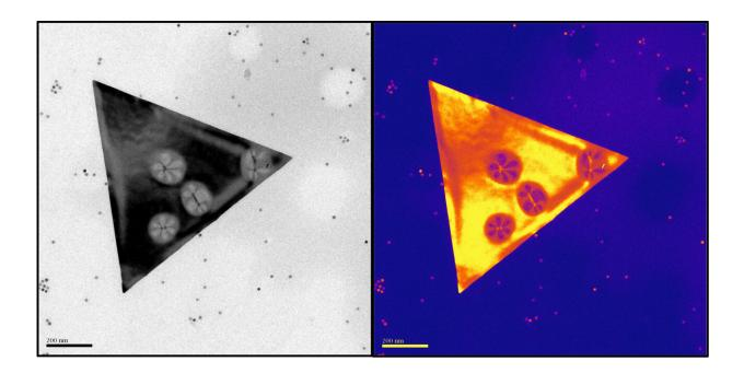
A transmission electron microscope image at left and a color map version at right highlights deformations in silver nanosheets laid over iron oxide nanospheres. Rice University scientists determined that van der Waals forces between the spheres and sheets are sufficient to distort the silver, opening defects in their crystalline lattices that could be used in optics or catalysis. Credit: The Jones Lab/Rice University
