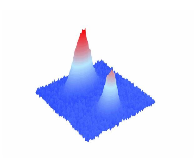
False-color image of a gas of potassium-rubidium polar molecules (left) becoming denser and colder in reaching a state called quantum degeneracy (right), in which the individual molecules' matter waves overlap to create an interdependent system. Credit: Ye Group/JILA
