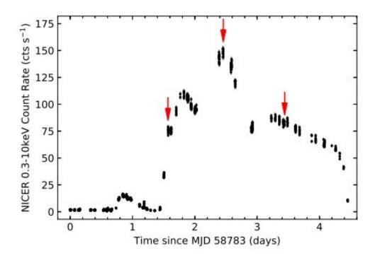
NICER long-term light curve of MAXI J1807+132 with 25 s time resolution in the 0.3–10 keV energy band. This section of the outburst contains the three thermonuclear X-ray bursts detected in October 2019. The X-ray burst data have been removed for clarity, and their onsets marked by arrows. Credit: Albayati et al., 2020.
