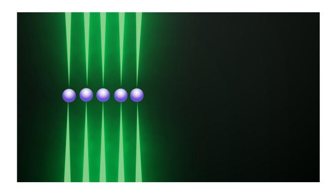
JILA's tweezer clock uses optical tweezers to confine and control many strontium atoms. Credit: NIST
