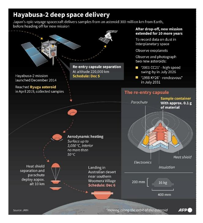
Graphic explaining how Japan's Hayabusa-2 space probe will drop off asteroid samples to Earth before starting a new mission
