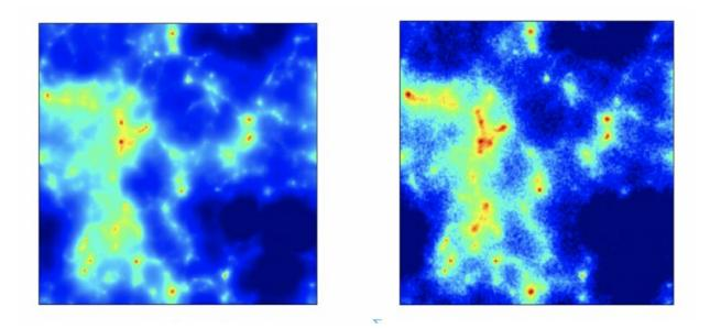
The researchers' Vlasov-Poisson simulation (left) predicts a smoother and less noisy density distribution of neutrinos compared to a traditional N-body particle simulation of Newtonian gravitational interaction (right). Credit: University of Tsukuba
