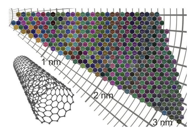
A color map illustrates the inherent colors of 466 types of carbon nanotubes with unique (n,m) designations based their chiral angle and diameter. Credit: Kauppinen Group/Aalto University
