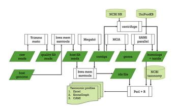
Lazypipe flowchart. Binaries and scripts are displayed in white, input and output files in green. Credit: University of Helsinki
