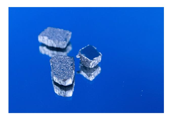
The Critical Materials Institute has developed a low-cost, high performance permanent magnet by drawing inspiration from an out-of-this-world source: ironnickel alloys in meteorites. Credit: U.S. Department of Energy Ames Laboratory
