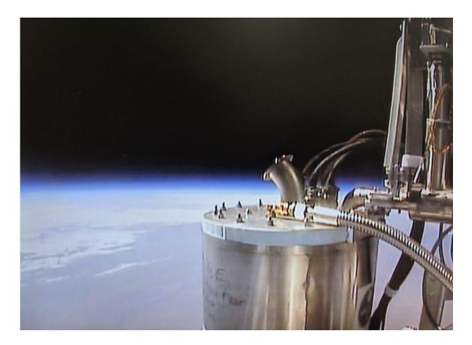
In-flight video still from BOBCAT during liquid helium transfer at an altitude of 130,000 feet. Credit: NASA
