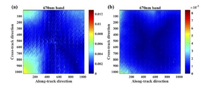
Fig. 2. Degree of polarization of the non-polarized light measured by each pixel of the 670nm band of the DPC. (a) Employing the original calibration parameters. (b) Employing the corrected calibration parameters. Credit: HUANG Chan
