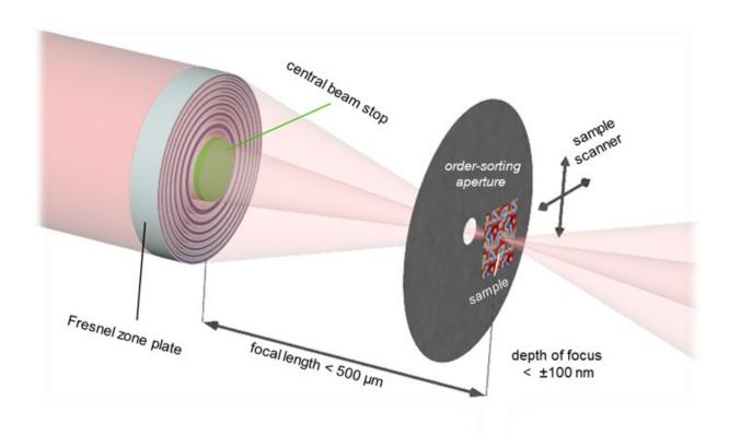
Fresnel zone plates are most commonly used as diffractive focusing elements in X-ray microscopy. In the Erlangen-STXM at the Paul Scherrer Institute, the beam is focused onto the specimen, which is raster-scanned at the highest precision. The transmitted beam is sensitive to local X-ray absorption, which probes elemental, electronic, magnetic, or chemical variations. Credit: Dr. Benedikt Rösner, Paul Scherrer Institute
