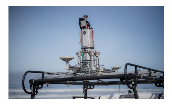
Truck-mounted sensor creates 3-D maps of beaches and cliffs to track erosion processes. Credit: Erik Jepsen/UC San Diego
