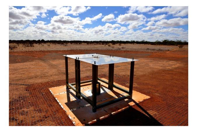
The Experiment to Detect the Global EoR Signature (EDGES) instrument. Credit: CSIRO, Author provided
