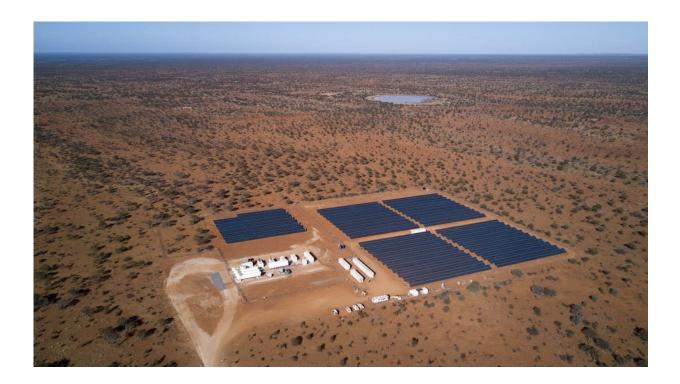
Aerial view of the MRO power station, which has an array of 5,280 solar panels and battery with RFI shielding. Credit: CSIRO, Author provided
