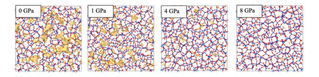
The voids (yellow) in silica glass become much smaller when the glass is quenched at higher pressures. Credit: Yongjian Yang, Penn State
