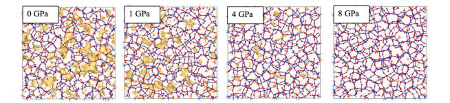
The voids (yellow) in silica glass become much smaller when the glass is quenched at higher pressures. Credit: Yongjian Yang, Penn State
