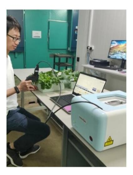
Portable leaf-clip Raman sensor being used at TLL to detect nutrient stress in leafy vegetables. Credit: Singapore-MIT Alliance for Research and Technology (SMART)
