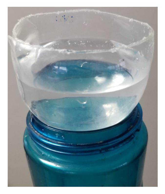
The prototype PLA cup developed by Kumho Polymer Science Professor Shi-Qing Wang, Ph.D., is transparent and super tough, and does not shrink when filled with boiling water. Credit: University of Akron
