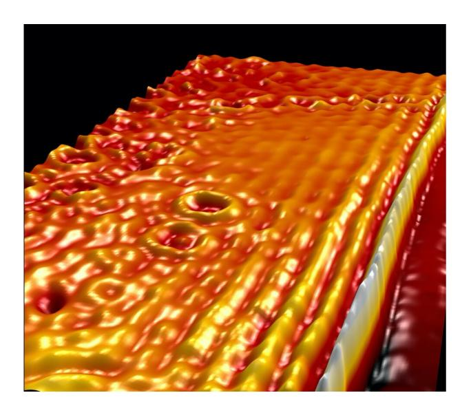
Massive work function-mediated charge transfer in graphene/?-RuCl3 heterostructures provides the necessary conditions for generating plasmon polaritons without electrostatic or chemical doping. The image depicts a
