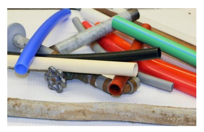
Some common types of drinking water pipes: Black plastic is HDPE; white is PVC; yellow is CPVC; red, maroon, orange, and blue are PEX; green is PP; and gray is polybutylene. The metal pipes are lead, iron and copper. Credit: Andrew Whelton/Purdue University, CC BY-ND
