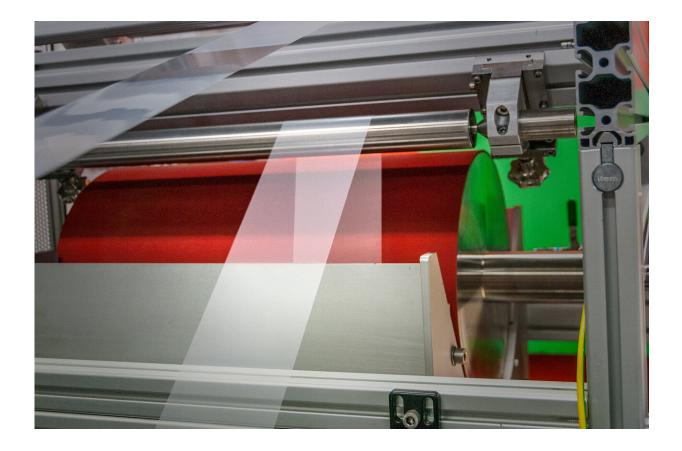
Aldyne system for continuous roll-to-roll functionalization, crosslinking and coating. Credit: Fraunhofer IST/Falko Oldenburg
