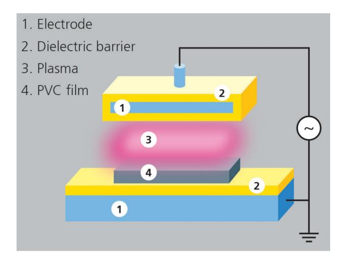
Experimental assembly for the DBD (dielectric barrier discharge) treatment of PVC films. Credit: Fraunhofer IST
