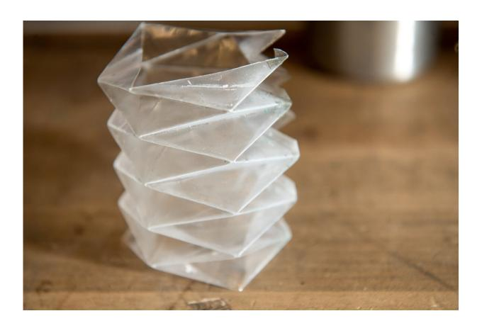
The researchers have developed an origami-inspired, folded plastic fuel bladder that doesn't crack at super cold temperatures and could someday be used to store and pump fuel. Credit: WSU
