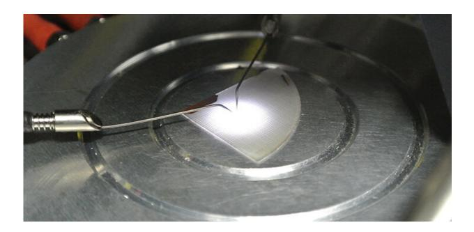
Monolithic LEDs emit a natural-white light without using phosphors. Credit: KAUST
