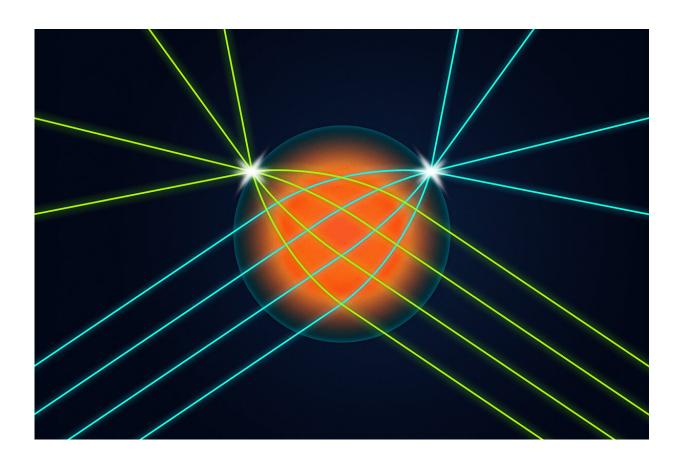
Illinois researchers developed a spherical lens that allows light coming into the lens from any direction to be focused into a very small spot on the surface of the lens exactly opposite the input direction. This is the first time such a lens has been made for visible light. Credit: Graphic by Michael Vincent
