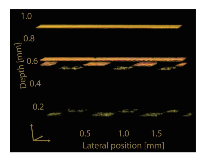
Researchers used entangled photons to increase the penetration depth of OCT for scattering materials. They demonstrated the technique by analyzing two alumina ceramic stacks containing laser-milled microchannels. The mid-infrared illumination allowed the researchers to capture depth information and to create a full 3D reconstruction of the channel structures (pictured). Credit: Aron
