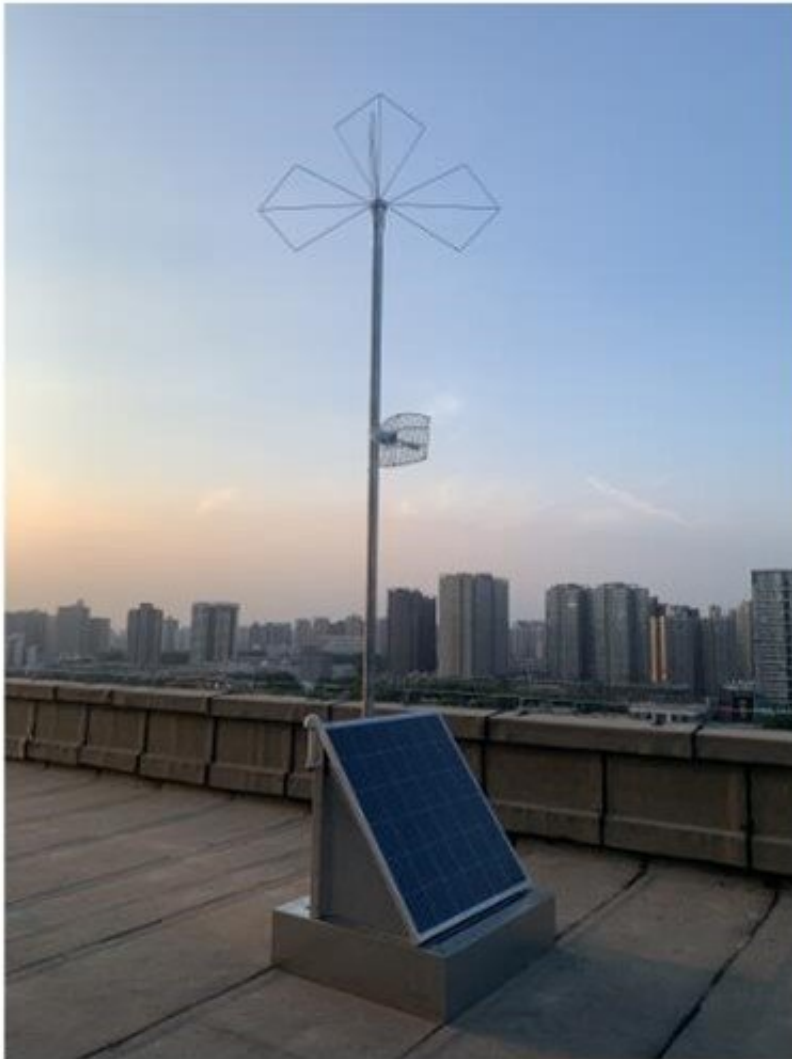
A prototype data collector and transceiver for the GRAND system. Credit: Sijbrand de Jong / GRAND Collaboration
