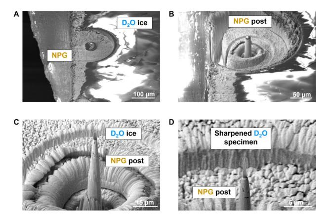
SEM images of in situ APT specimen preparation of an ice sample on NPG (nanoporous gold). (A) The 200- and 75- $\mu$ m ion beam annular patterns for outer and inner diameters, respectively, were made on the ice/NPG sample. (B) The ice/NPG pillar was milled until the height of the Au post reached
