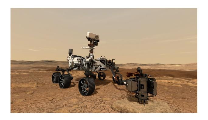
In this illustration, NASA's Mars 2020 rover uses its drill to core a rock sample on Mars. Credit: NASA/JPL-Caltech
