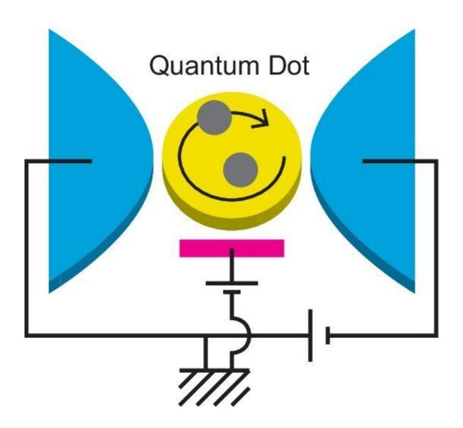
A schematic illustration of a nanoscale circuit. A quantum dot (the yellow part) is connected to two lead electrodes (the blue parts). Electrons tunneling into the quantum dot from the electrodes interact with each other to form a highly correlated quantum state, called "Fermi liquid". Both nonlinear electric current
