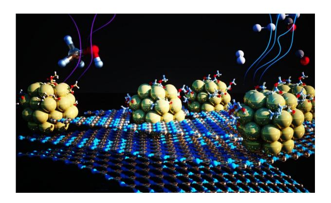
An illustration of the 2D boron nitride substrate with imperfections that host tiny nickel clusters. The catalyst aids the chemical reaction that removes hydrogen from liquid chemical carriers, making it available for use as a fuel. Credit: Jeff Urban/Berkeley Lab
