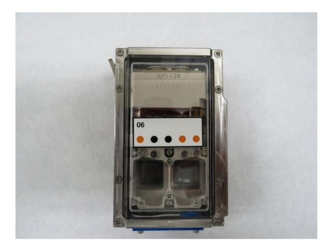
A preflight view of BioAsteroid Experiment Unit where the BioAsteroid investigation is performed integrated into the Experiment Container for the BioAsteroid investigation. Each Experiment Unit has two culture chambers. Credit: ESA
