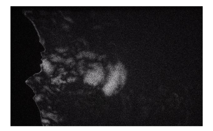
The new imaging technique has been used to capture the exhaled breath of a person speaking. This is a demonstration of the published imaging technique that is being further investigated. The imaging shows only the temperature change associated with exhaled breath, which does not necessarily reflect the movement of viral particles contained in the breath. Credit: Thomas Moore, Rollins College
