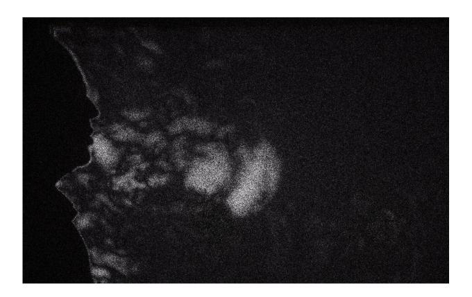
The new imaging technique has been used to capture the exhaled breath of a person speaking. This is a demonstration of the published imaging technique that is being further investigated. The imaging shows only the temperature change associated with exhaled breath, which does not necessarily reflect the movement of viral particles contained in the breath. Credit: Thomas Moore, Rollins College
