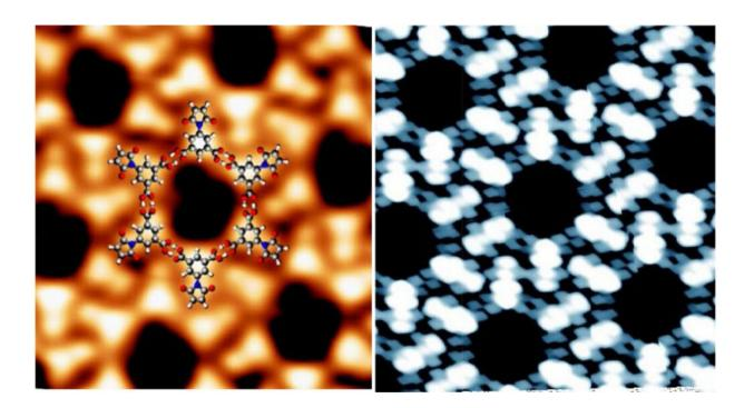
Magnified experimental and simulated scanning tunnelling microscopy images of the molecule used (maleimide derivative-BCM) network on graphene. Credit: INRS
